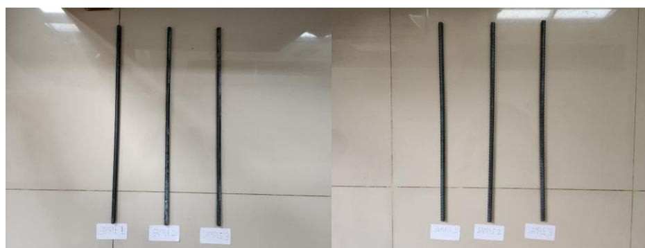
Figure 1. Reinforced Concrete Sample Plain Ø10 mm (Left) and Threaded Rebar D10 mm (Right)
