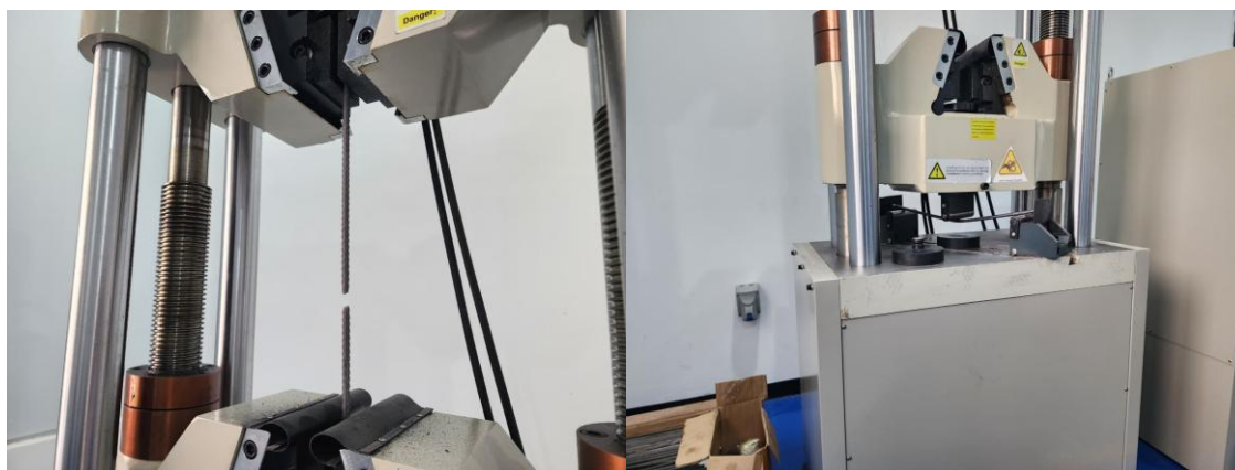
Figure 2. Implementation of Tensile Test (Left) and Bend Test (Right) Using UTM
