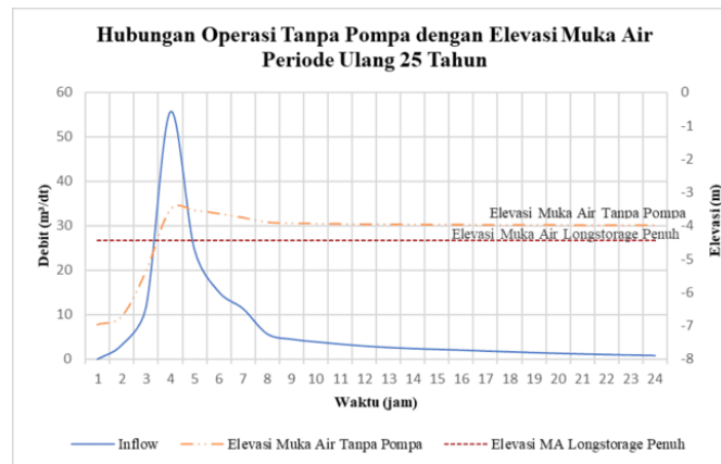
Figure 12. Relationship Between Non-Pumped Operation and Water Surface Elevation in the Long-Storage Unit for the 25-Year Return Period
