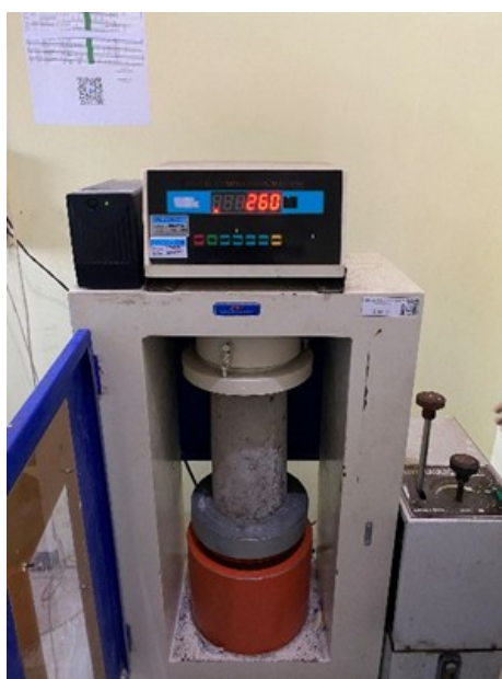
Figure 4. Compressive Strength Test Visualization
