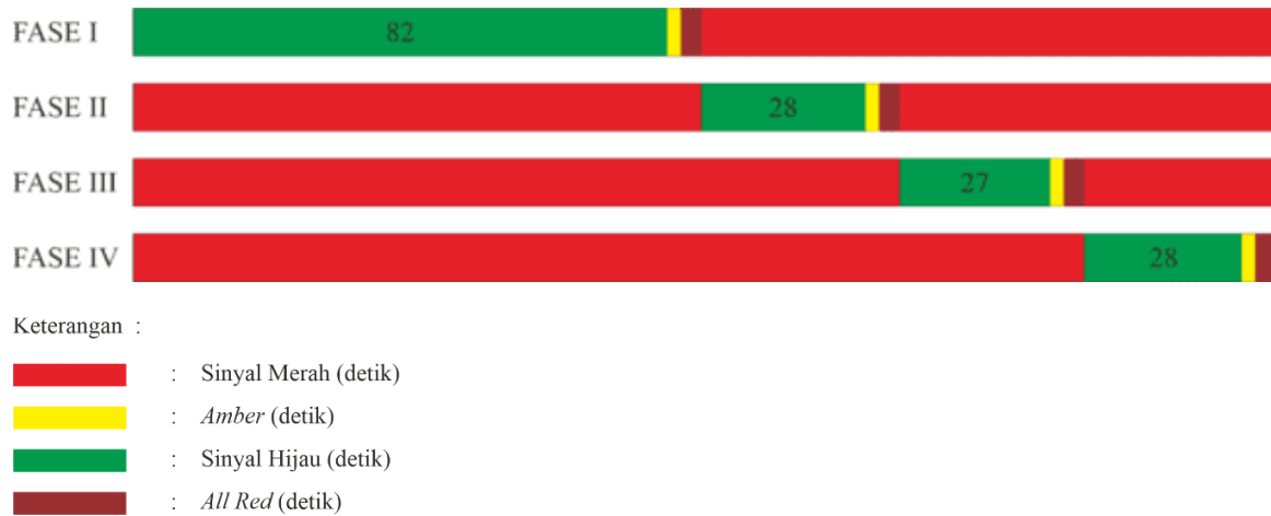
Figure 5. Phase Diagram of Gayamsari Intersection Active Afternoon Peak Hour
