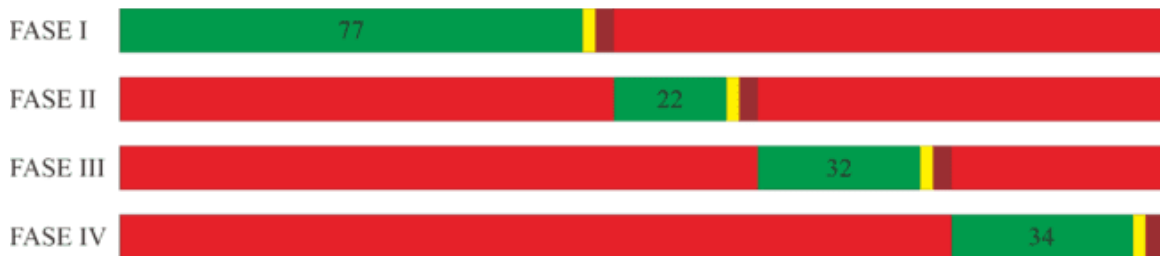
Figure 2. Phase Diagram of Gayamsari Intersection Active Morning Peak Hour
