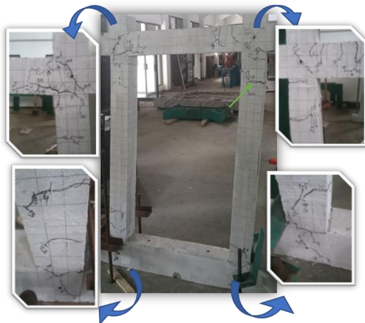
Figure 7. Testing Documentation of Portal without Brace
