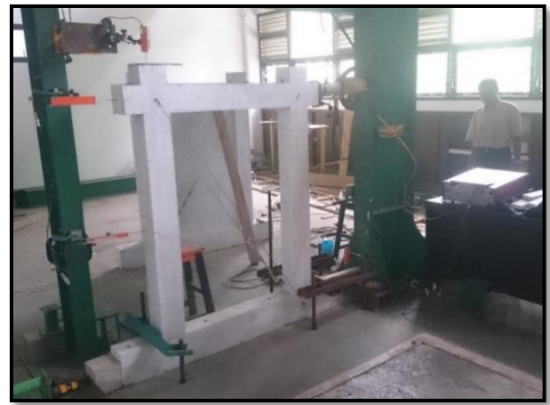
Figure 5. Placement of Test Objects Before Testing on Loading Frame
