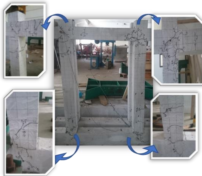
Figure 9. Documentation of Portal Testing with Braces
