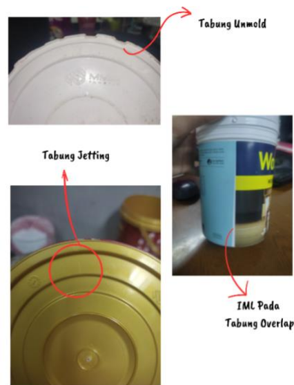
Figure 1. Defect in Tube No. 10 VC TM
