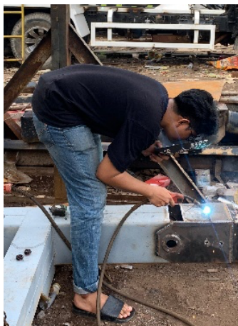
Figure 2. Metal welding process
