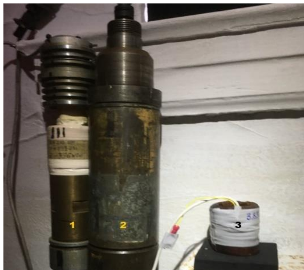
Figure 1. – MIG-3V geophone sensor, 2 – MIG-3V geophone,
