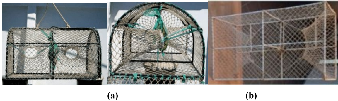
Figure 3. (a) Trap with two entrances side by side and (b) trap with two entrances in opposite directions ( Catalogue of fishing gear in the Mediterranean, n.d. )
