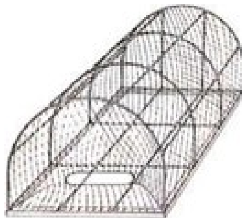
Figure 2. Spiny lobster pots design in east coast of Australia (FAO, 1972)
