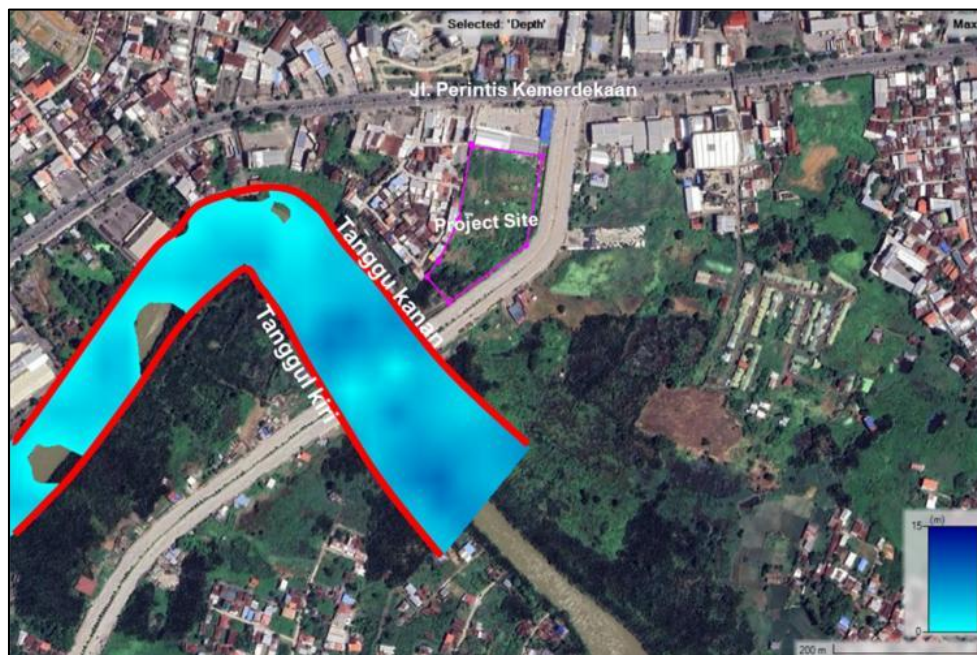
Figure 4 Hydraulic Simulation Results with a 2.5 m High River Embankment,
