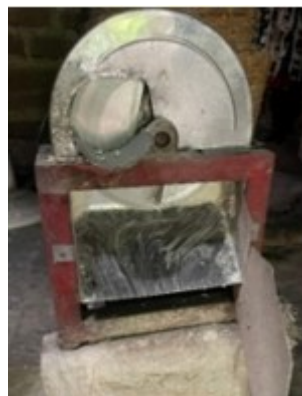
Figure 2. Cassava Cutting Tools for the Pitulikur MSME from the Ministry of Manpower
